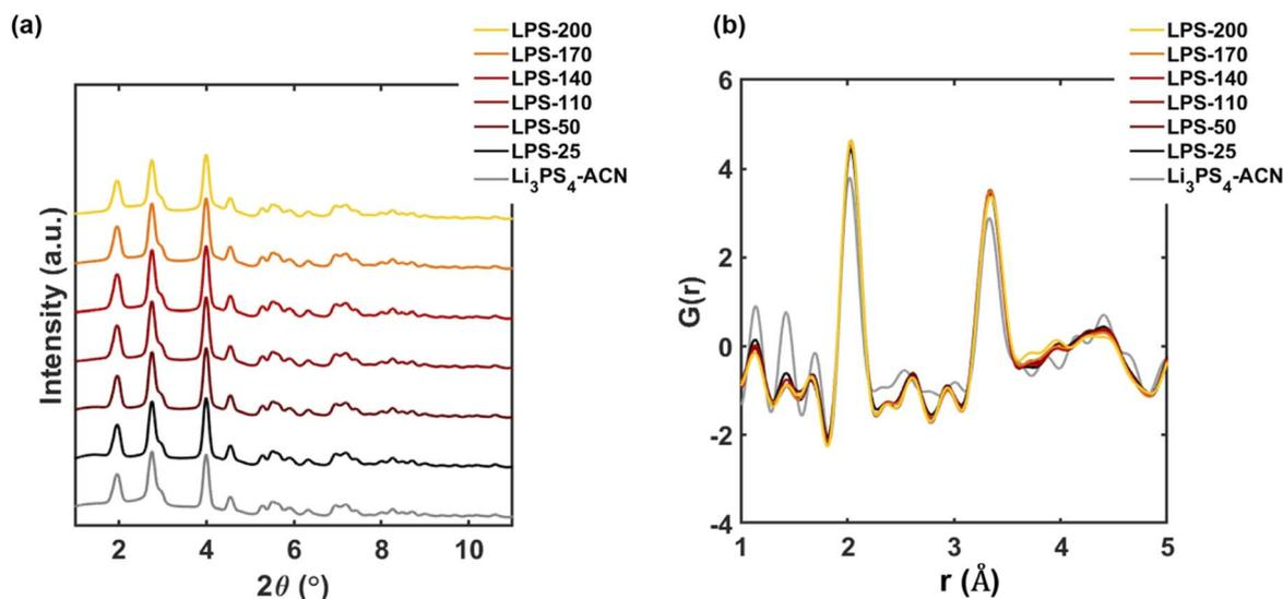
Fig. 3 Synchrotron diffraction Bragg data (a) and reduced PDFs (b) of SEs after annealing at temperatures below 200 °C. The data of the pure  $\text{Li}_3\text{PS}_4\text{-ACN}$  crystalline complex is also provided for comparison.
